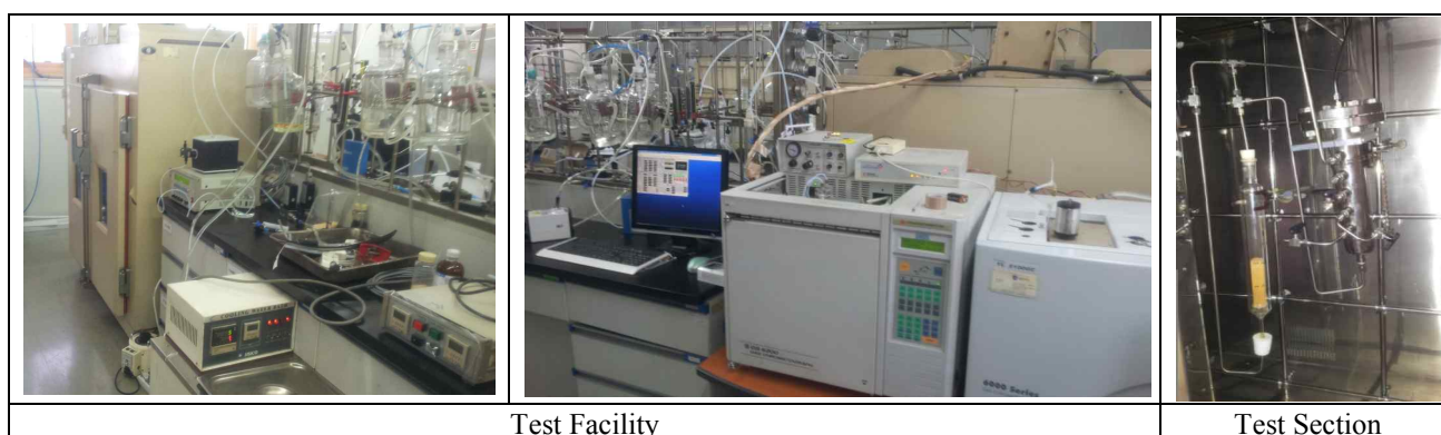
Figure 1. Organic Iodide Removal Test Facility and Test Section.
