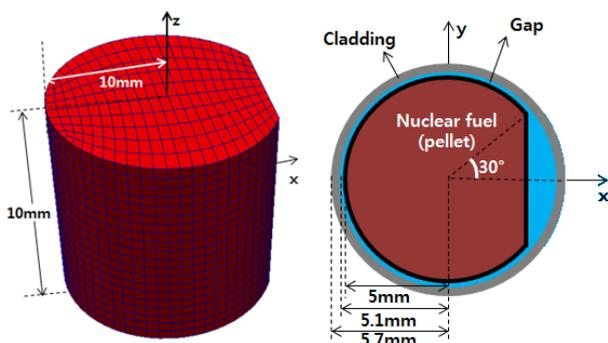
Fig. 2. Generation of elements for MPS simulation
