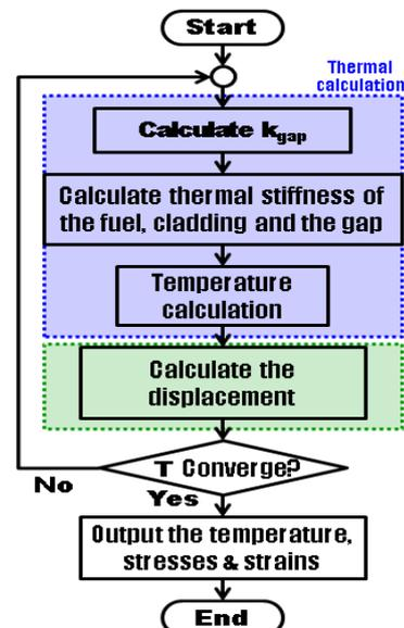
Fig. 1. Flowchart of 3D thermo-mechanical calculation
