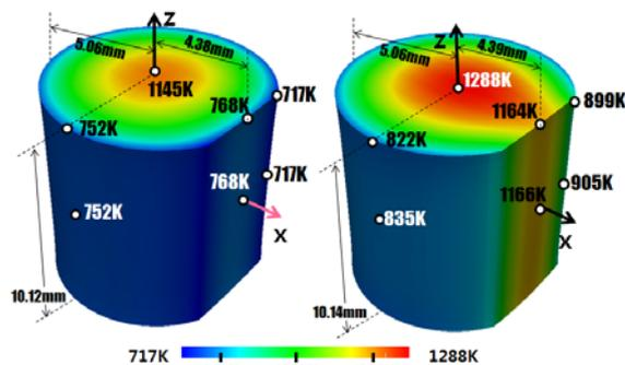
Fig. 3. Temperature distribution of uniform gap conductance (left) and 3D dynamic gap conductance (right) for MPS simulation
