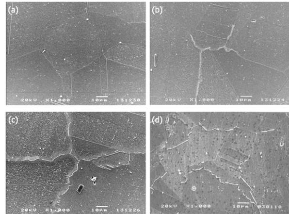
Fig. 9 Grain boundary morphologies and intergranular Cr carbide precipitations in Alloy 690-3C attained at (a) 1000 °C, (b) 990 °C, (c) 900 °C, and (d) 800 °C during controlled cooling with a cooling rate of 0.5 °C/min
