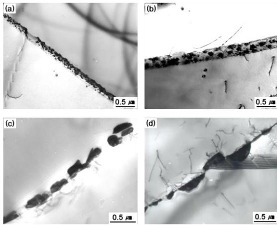
Fig. 4 Carbide precipitation on random high-angle grain boundaries in 690-2C after thermal treatments for (a) 0.1 hr, (b) 1 hr, (c) 10 hr, and (d) 100 hr at 720 °C
