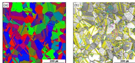
Fig. 1 EBSD results showing the grain boundary characteristics of 690-2C: (a) orientation image map and (b) grain boundary map denoted by the CSL model
