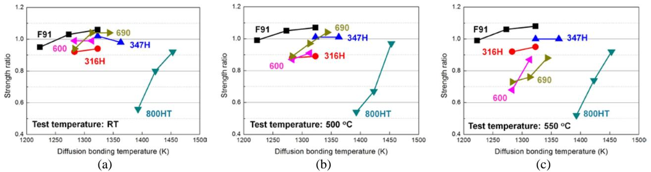
Fig. 1. Influence of the diffusion bonding temperature on the strength ratio at (a) RT, (b) 500 °C, and (c) 550 °C.
