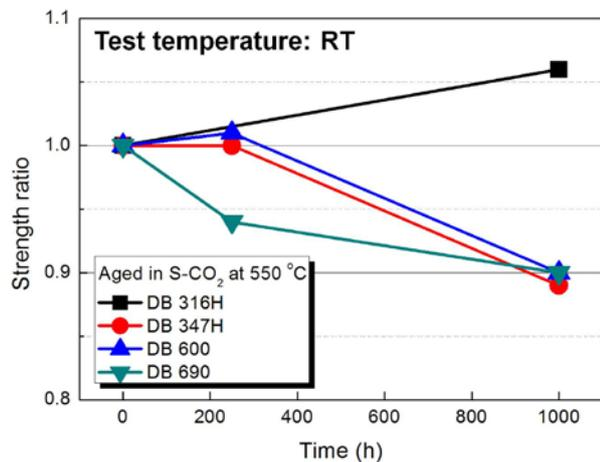
Fig. 2. Strength ratio of the ultimate tensile strength of the as-bonded and aged in S-CO<sub>2</sub> at 550 °C.
