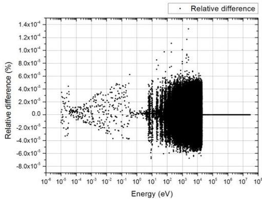
Fig. 1. Relative difference of the  $^{238}\text{U}$  cross sections at 600K calculated by the McCARD SIGMA1 module
