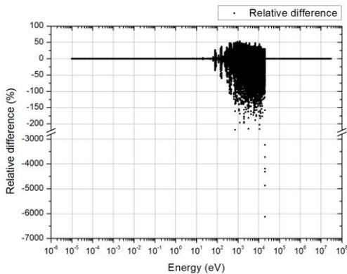
Fig. 2. Relative difference of the  $^{238}\text{U}$  cross sections at 600K calculated by the McCARD LHDB module using 0K data
