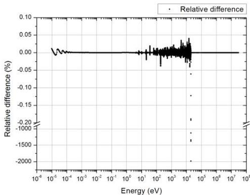
Fig. 3. Relative difference of the  $^{238}\text{U}$  cross sections at 600K calculated by the McCARD LHDB module using 300K data
