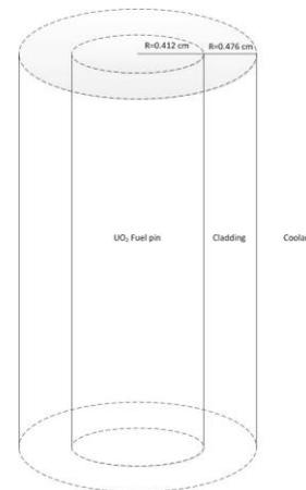
Fig. 4. Geometry of a  $\text{UO}_2$  fuel pin cell problem
