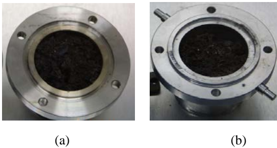
Fig. 2. Photographs of uranium deposits (a) in a sieve and (b) in a crucible
