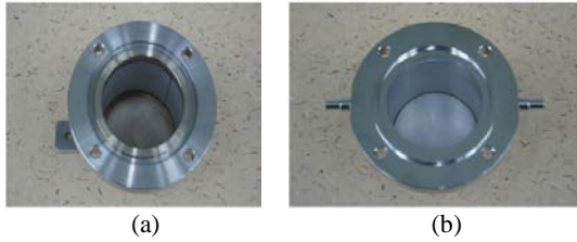
Fig. 1. Photographs of (a) a sieve for the solid-liquid separation and (b) a crucible for the integrated sieve-crucible assembly.
