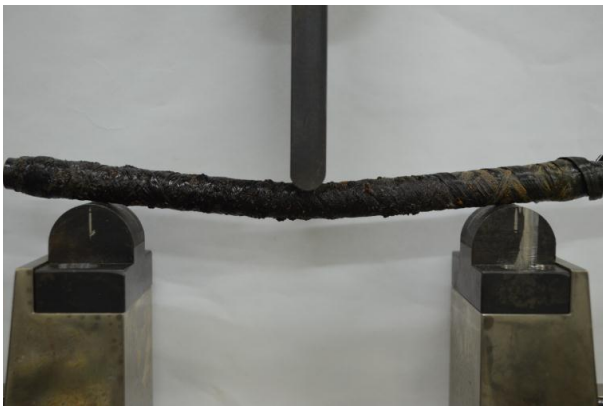
Fig. 3. Specimen loaded on a three-point bend test.
