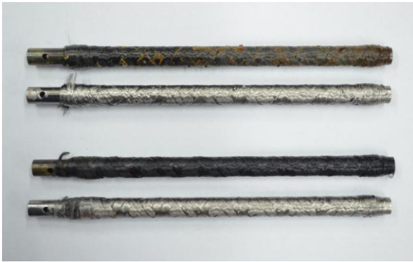
Fig. 2. Specimens for a three-point bend test that were fabricated differently: i) wet process, ii) wet process followed by a Zr surface coating, iii) wet process with a Zr interphase coating, and iv) wet process with a Zr interphase coating followed by a Zr surface coating.
