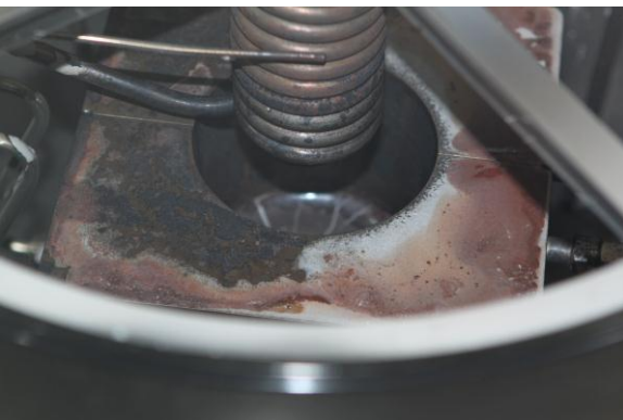
Fig.4. Fabricated salt by mold of pelletizer at 200°C
