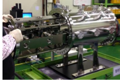
Fig. 6. Assembly of the electrode structure and the vacuum chamber.
