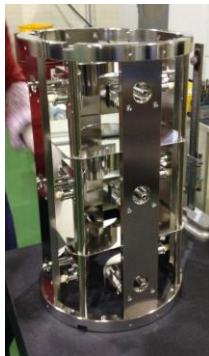
Fig. 5. Assembled electrodes structure of the ESQ triplet
