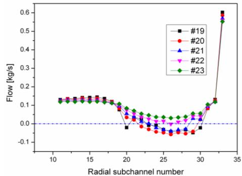
Figure 5. Axial flow distribution for the 54-middle blockage
