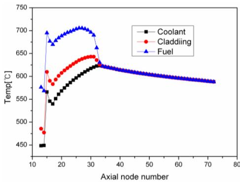
Figure 3. Axial temperature distribution for the 24-middle blockage
