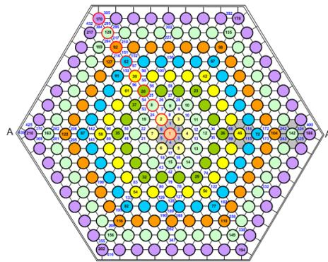
Figure 1. Numbering of the sub-channels and fuel rods, and blockage positions for the analysis
