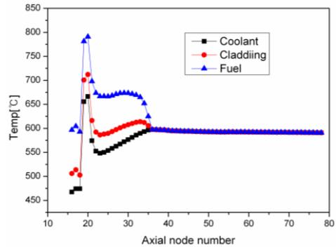
Figure 3. Axial temperature distribution for the 54-middle blockage
