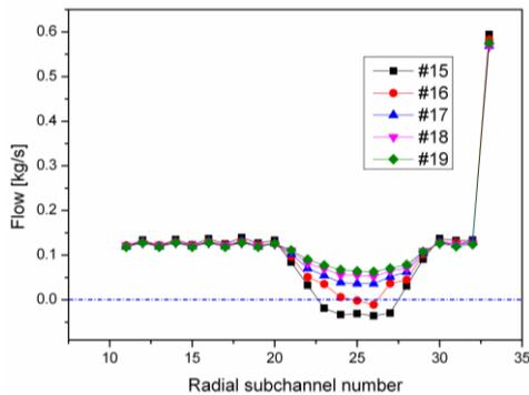
Figure 4. Axial flow distribution for the 24-middle blockage
