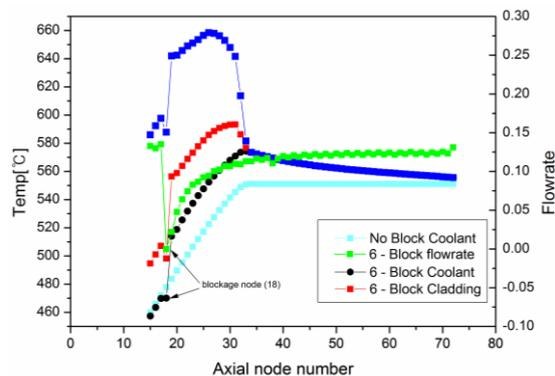
Figure 2. Axial temperature distribution for the 6-middle blockage
