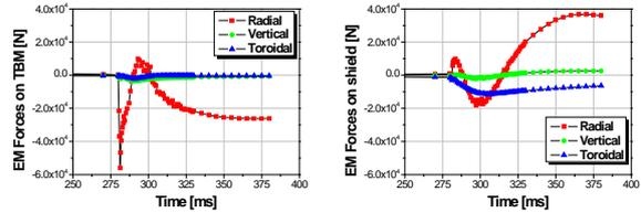
Fig. 5 Radial, vertical and toroidal component of electromagnetic force on TBM and shield during major disruption exponential 16ms
