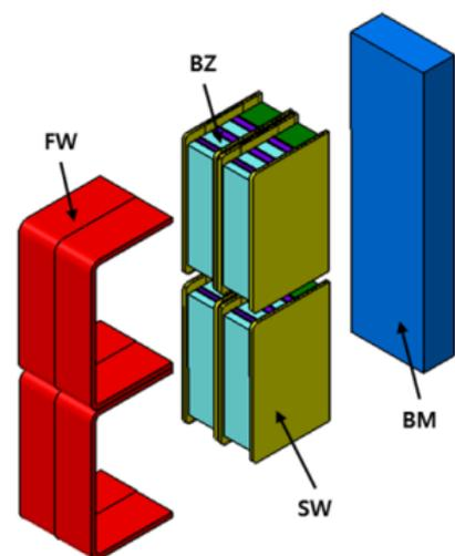
Fig. 1 The model of HCCR TBM
