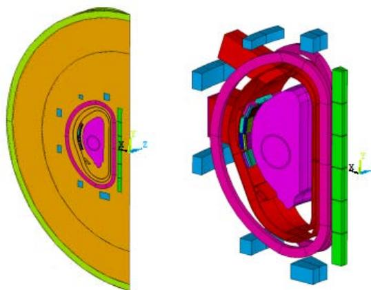
Fig. 2 Full geometry model for the 20 degree Sector of ITER and except the vacuum region
