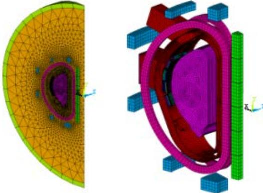
Fig. 3 Full finite element model for the 20 degree sector model and except the vacuum region
