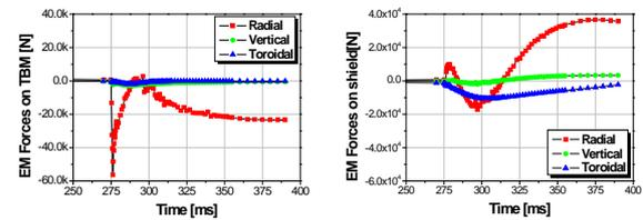
Fig. 6 Radial, vertical and toroidal component of electromagnetic force on TBM and shield during major disruption exponential 22ms
