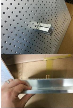
Fig. 2. The photograph of fabricated faraday cup array
