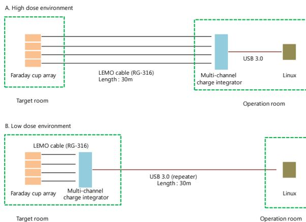
Fig. 4. The Schematic views of current measurement system depending on the target room environment. A. High dose environment, B. Low dose environment.
