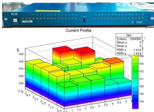
Fig. 3. 32-ch charge integrator (upper panel) and 2-D profile by measuring the charge integrator
