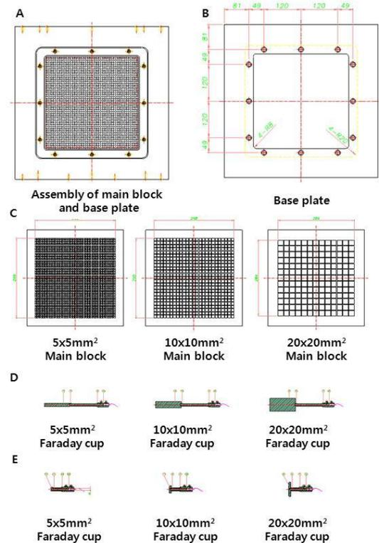
Fig. 1. Schematic drawing of faraday cup array A. assembly of main block and base plate, B. base plate, C. Main block, D. Faraday cup for 100 MeV proton beam, E. Faraday cup for 20 MeV proton beam.
