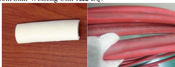
Figure 2. The 'tested cable' from Han-UI NPP Unit 3&4
