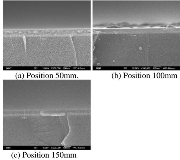
Fig. 4. Show the SUS 304 coated Si-wafer cross section images (FE-SEM).
