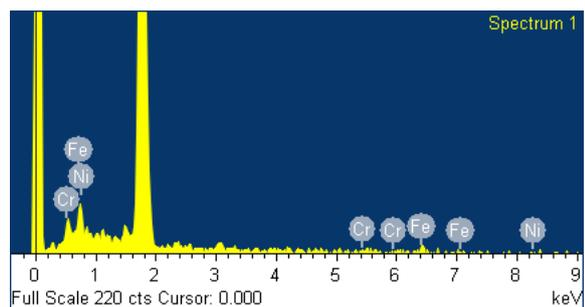
(b) Cr and SUS 304 deposition metal component ratio according to current density  $160 \mu\text{A}/\text{cm}^2$ .
