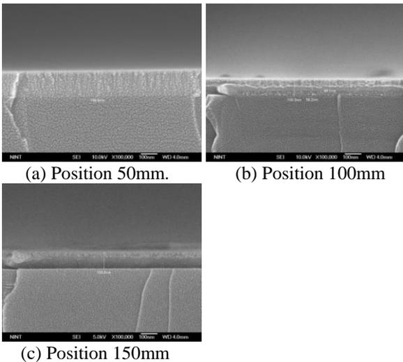
Fig. 3. Show the Cr coated Si-wafer cross section images (FE-SEM).
