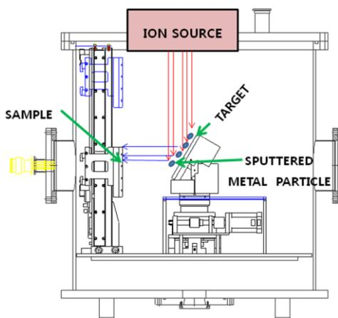
Fig. 1. A schematic diagram of the ion beam sputtering deposition system. The line indicates the flow of argon ions.
