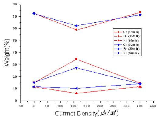
(a) Cr and SUS 304 deposition metal component ratio according to current density.
