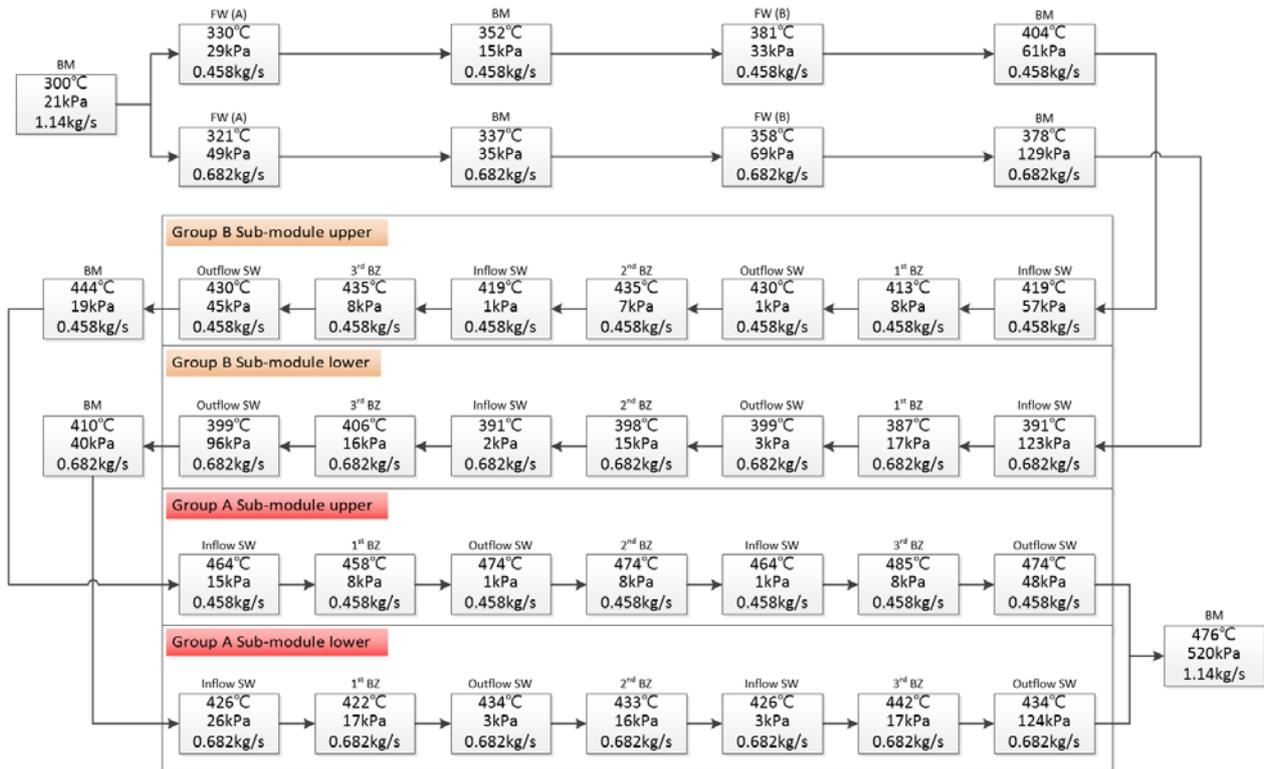
Fig. 4. Flow scheme and coolant information by integrated analysis.
