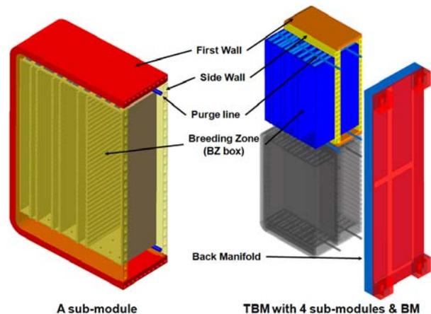
Fig. 1. Concept of KO HCCR TBM and its sub-modules.
