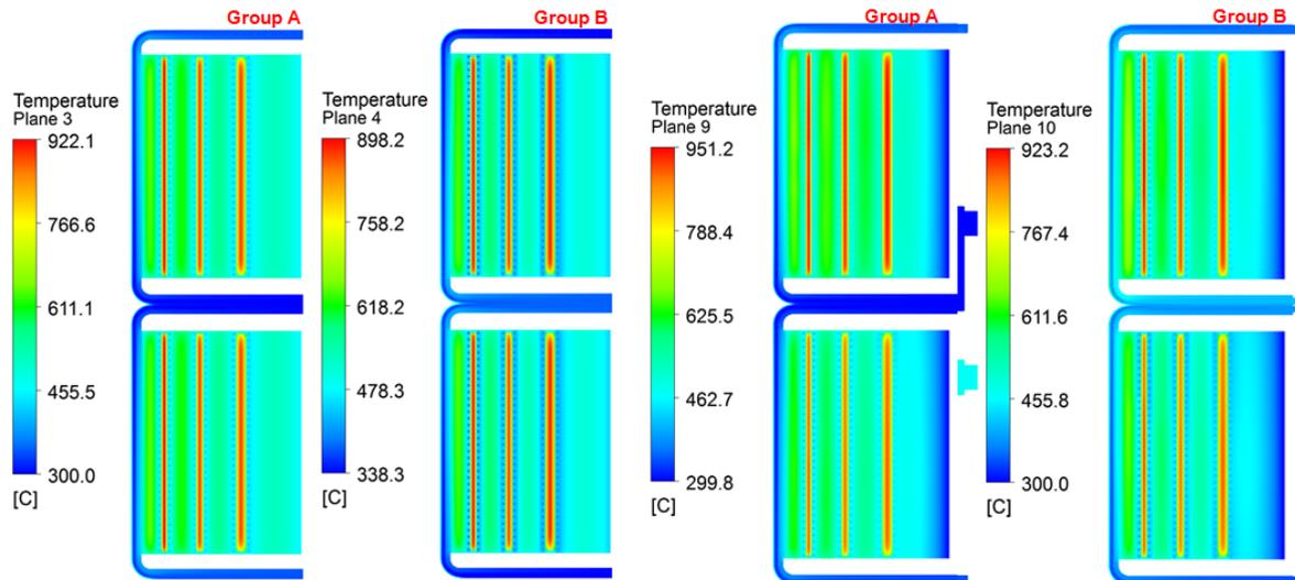
BZ with FW solid simulation, left side view and local range
