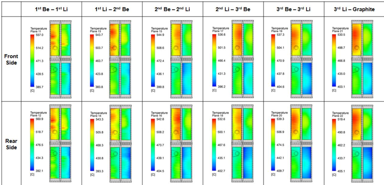
Fig. 11. BZ structure temperatures according to the location
