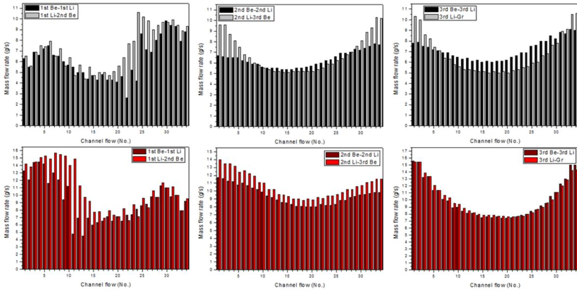
Fig. 7. Flow distribution in the BZ plate.
