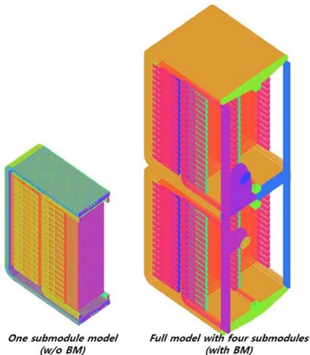
Fig. 3. Integrated models and meshes for submodule and whole model
