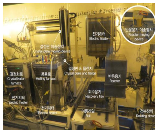
Fig. 2 Engineering-scale layer-melt crystallization equipment for the purification of LiCl waste salt.
