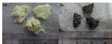
Fig. 1. As synthesized granular porous bismuth (a) not treated with hydrogen and (b) treated with hydrogen.
