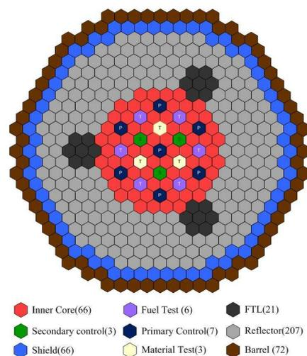
Fig. 1. Radial core layout of MESOF
