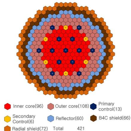
Fig. 4. Radial core layout of small-sized KALIMER-300
