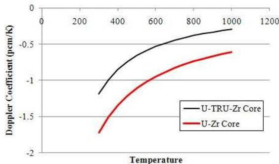
Fig. 2. Comparison of the Doppler coefficient between U-Zr and U-TRU-Zr core
