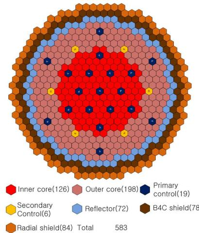
Fig. 3. Radial core layout of KALIMER-600
