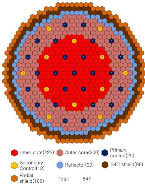
Fig. 5. Radial core layout of large-sized KALIMER-1200
