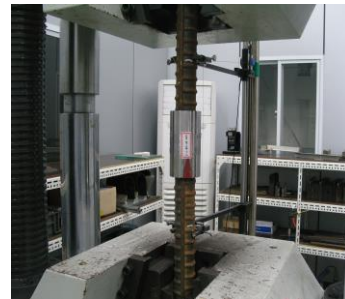
Fig. 3 Test set-up of the tensile test
