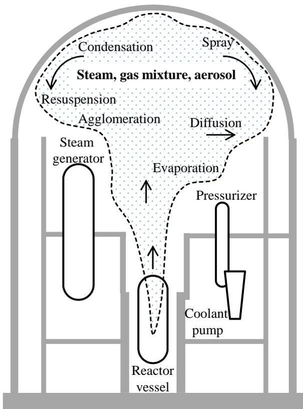
Fig. 1. Complicated phenomena in containment building under a severe accident
