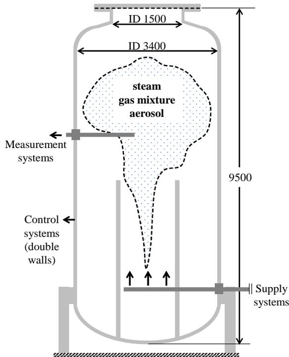
Fig. 2. Schematic of KAERI test facility
