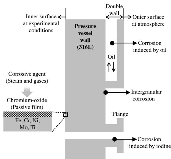
Fig. 3. Corrosion in large-sized pressure vessel
