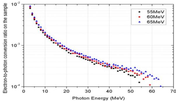
Figure 3: Electron-to-photon conversion ratio calculated by MCNPX as function of photon Energy.
