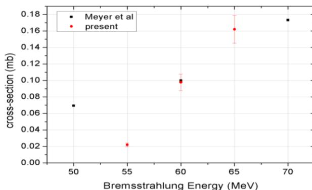
Figure 4: The cross-section of  $^{27}\text{Al}(\gamma, 2\text{pn})^{24}\text{Na}$  reaction induced by bremsstrahlung comparing with data of Meyer et al.
