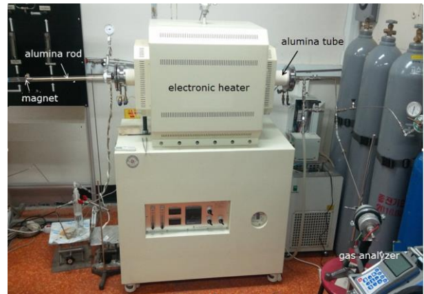
Fig. 1. Apparatus (tube furnace) for high temperature oxidation of Zr alloys.
