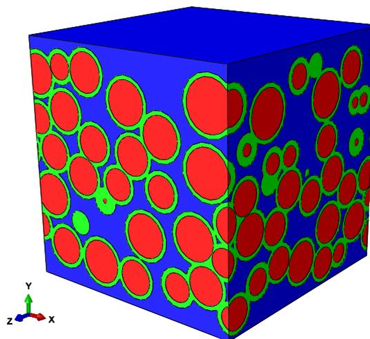
Fig. 1. Model of  $300 \times 310 \times 300 \mu\text{m}$  with a Volume Fraction of 40 vol% and an Interaction Layer Thickness of  $5 \mu\text{m}$
