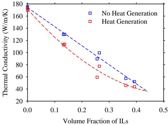
Fig. 5. The Effects of the Heat Generation on the Thermal Conductivity of Dispersion Fuel when the U-Mo is 20 vol%.
