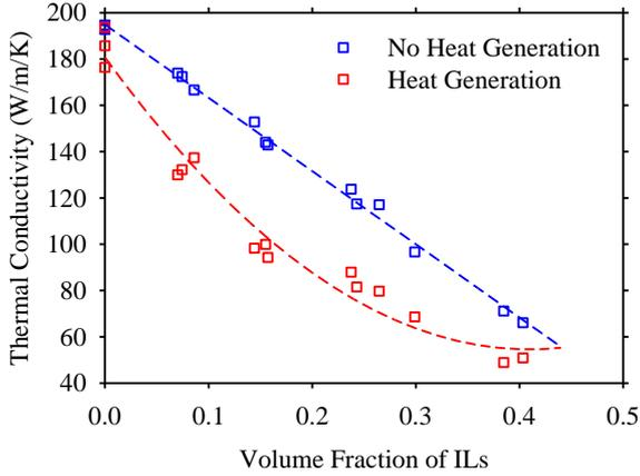
Fig. 4. The Effects of the Heat Generation on the Thermal Conductivity of Dispersion Fuel when the U-Mo is 10 vol%.
