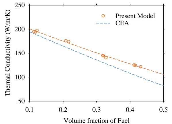
Fig. 3. Effective Thermal Conductivity Comparison between Present Model and CEA Equation.
