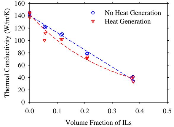
Fig. 7. The Effects of the Heat Generation on the Thermal Conductivity of Dispersion Fuel when the U-Mo is 30 vol%.
