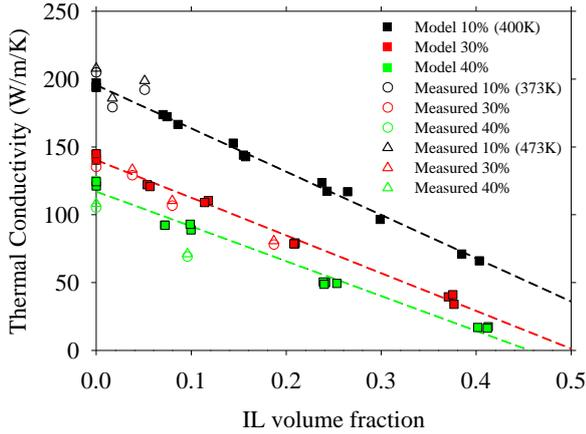
Fig. 2. Thermal Conductivity Comparison with Measured Data on U-10wt%Mo Dispersion Fuel Reported by Lee [6].
