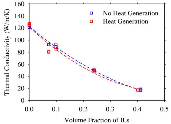
Fig. 8. The Effects of the Heat Generation on the Thermal Conductivity of Dispersion Fuel when the U-Mo is 40 vol%.
