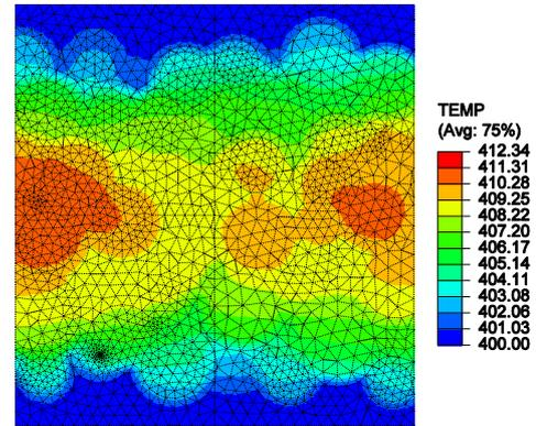
Fig. 9. The Temperature Distribution of the Dispersion Fuel with a Volume Fraction of 40 vol% and an Interaction Layer Thickness of 9  $\mu\text{m}$
