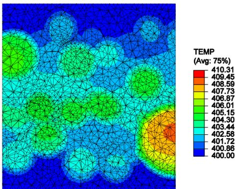
Fig. 6. The Temperature Distribution of the Dispersion Fuel with a Volume Fraction of 20 vol% and an Interaction Layer Thickness of 13  $\mu\text{m}$
