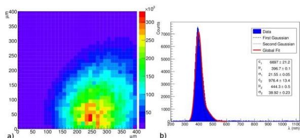
Fig. 4 IBIL map (a) and spectrum in highest detection sensitivity pixel (b) for Cu-doped fiber
