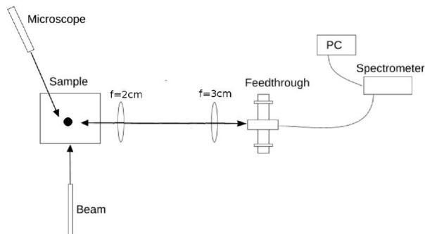
Fig. 3 Experimental setup for IBIL optical test
