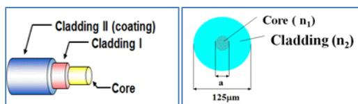
Fig. 1 Structure of Optical Fiber
