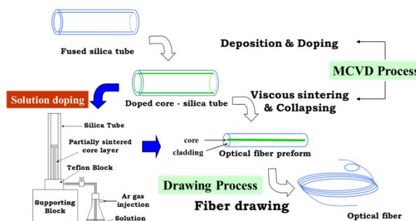
Fig. 2 Fabrication process of the optical fiber preform
