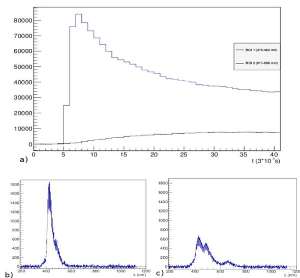
Fig. 5 a) Changes in intensity of IBIL peaks in relationship with time of proton microbeam irradiation; b) IBIL spectrum at the beginning of irradiation; c) IBIL spectrum after irradiation.
