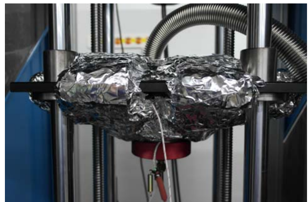
Fig. 2. The upper torr seal which is wrapped by coil heaters and covered by insulators.
