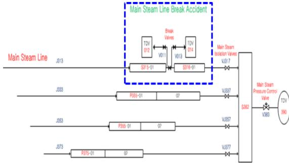
Fig. 3. Nodalization scheme of the main steam line break system
