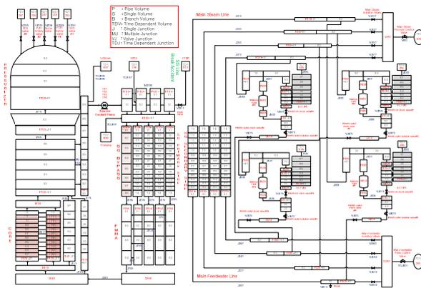
Fig. 1 MARS-KS nodalization scheme for SMART-SDA
