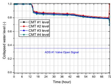
Fig. 12. Core Makeup Tank (CMT) collapsed water level
