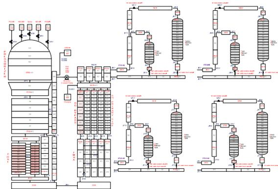
Fig. 2. MARS-KS nodalization scheme for SMART-PSS
