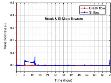
Fig. 6. Break & SI flow
