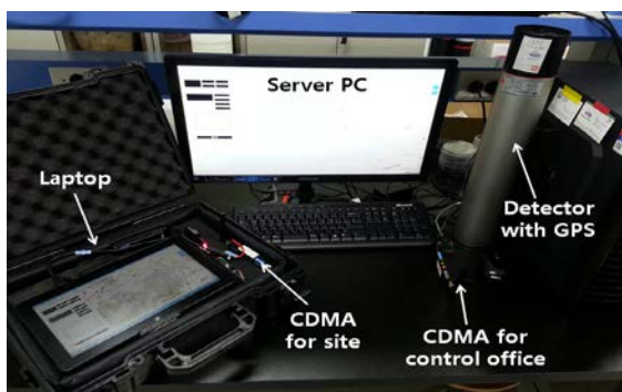
Fig. 1. Components of Radiation Distribution Monitoring System
