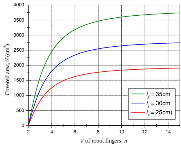
Fig. 9. Covered area of a PoFASS along the number of robot fingers.
