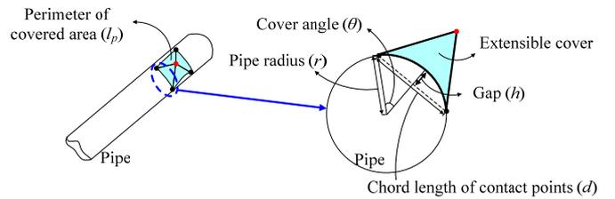
Fig. 4. Definition of the gap and parameters.
