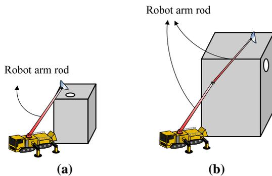
Fig. 10. Inaccessible leakage points of a PoFASS for the case of (a) one robot arm rod and (b) two robot arm rods.
