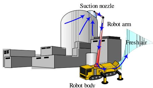
Fig. 1. Overview of a portable filtered air suction system [3].
