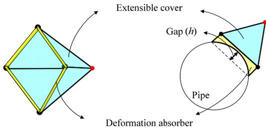
Fig. 7. Conceptual schematic of the deformation absorber.
