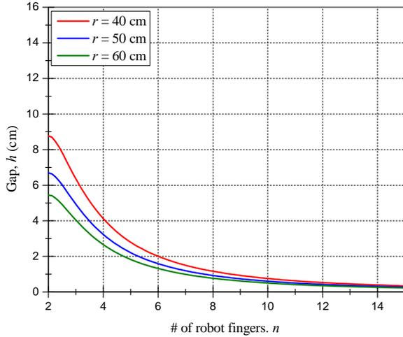
Fig. 6. The gap of the flexible robot suction nozzle along the number of robot fingers.
