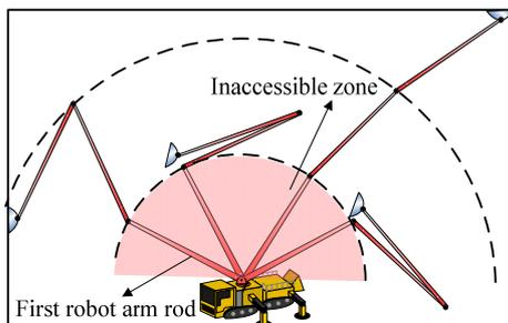
Fig. 11. Range of inaccessible zone of a PoFASS.
