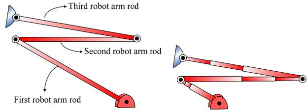
Fig. 12. Conceptual schematic for three robot arm rods (a) with a single stage and (b) with multi-stage.
