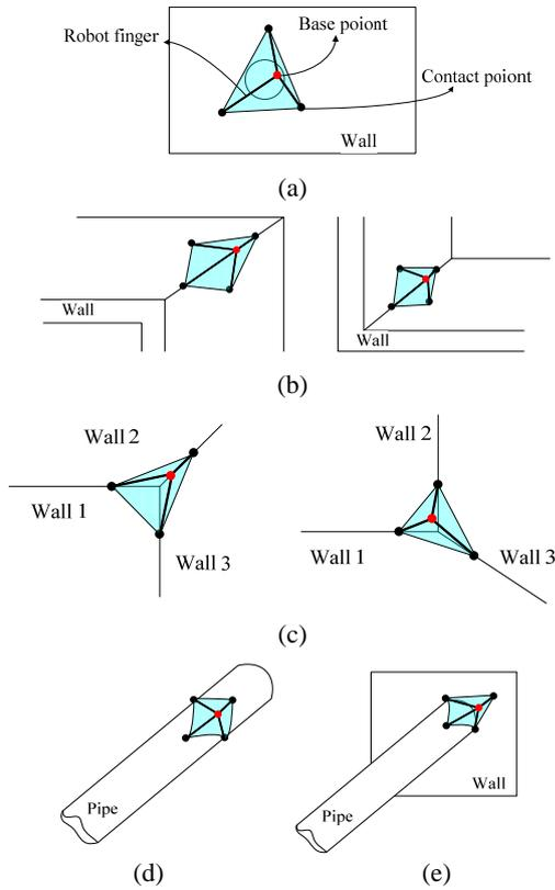
Fig. 3. Minimum number of robot fingers to cover the leakage point [3] in case of (a) side of wall, (b) corner of walls, (c) vertex of walls, (d) side of pipe, and (e) joint of pipe and wall fractures.
