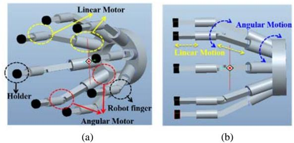
Fig. 2. Configuration of the flexible robot suction nozzle [3].
