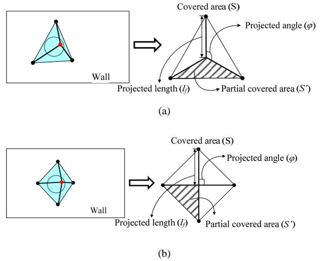
Fig. 8. Modeling of covered area in case of (a) three robot fingers and (b) four robot fingers.
