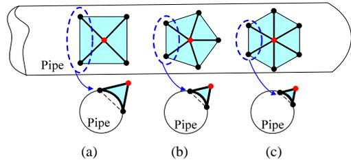
Fig. 5. Comparison of gaps along the number of robot fingers in case of (a) four robot fingers, (b) five robot fingers, and (c) six robot fingers.
