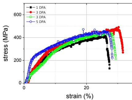
Fig. 2. Stress-strain curve for proton irradiated sample.
