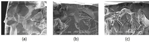
Fig. 3. SEM image on fracture surface for a) 1 DPA, b) 3 DPA and c) 5 DPA after SSRT test in PWR primary water.
