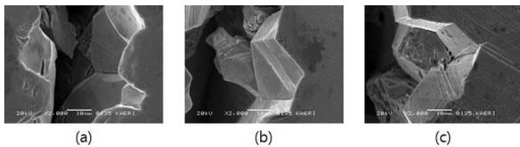
Fig. 4. SEM image on gage surface for a) 1 DPA, b) 3 DPA and c) 5 DPA after SSRT test in PWR primary water.
