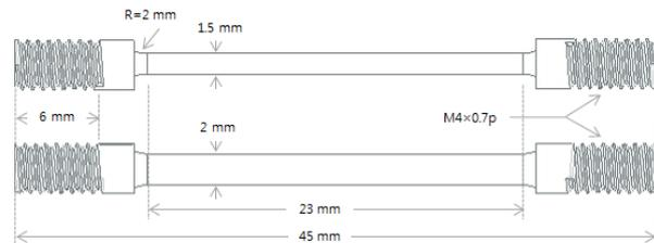
Fig. 1. Schematic of tensile specimen.
