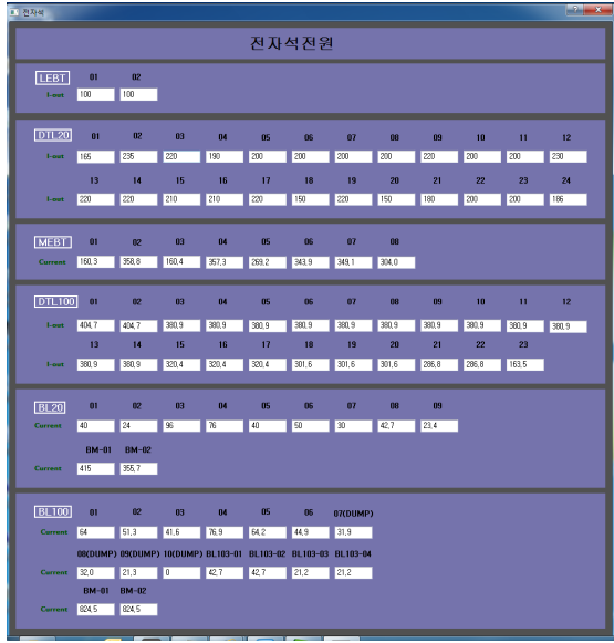
Fig. 3. The input monitor for the quadrupole current in the beam simulator.
