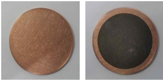
Fig. 2. 2\mu\text{m} titanium target fabricated by evaporation instrument for fast neutron production
