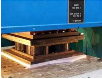
Figure 4. An isolation system for performing a dynamic test
