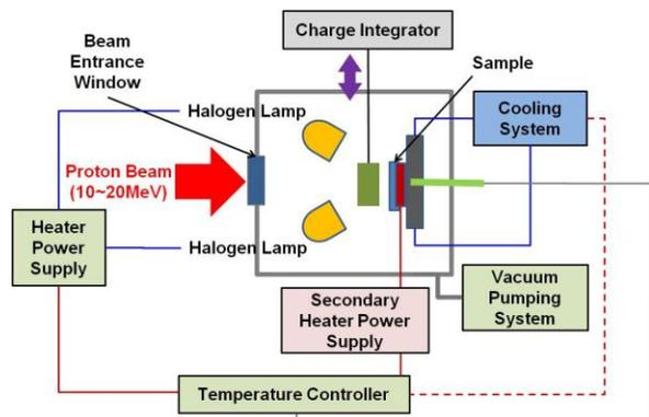
Fig. 2. Design concept of proton beam irradiation chamber system.
