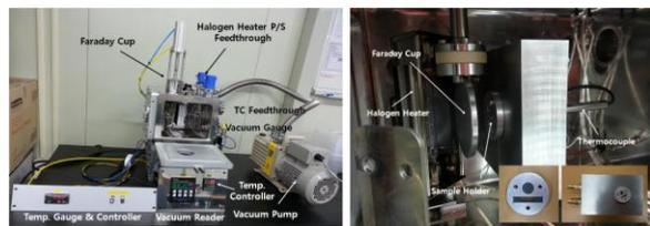
Fig. 3. Proton beam irradiation system.
