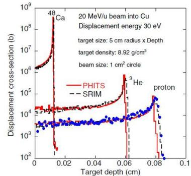
Fig. 1. SRIM code calculation results (filled dot) compared to others; depth dependence of the displacement cross section is shown for a 5 cm radius and 0.1 cm thick copper and tungsten target irradiated by 20 MeV/u proton, <sup>3</sup>He and <sup>48</sup>Ca beams.
