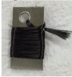
Figure 3. SiC fiber is wound around the Zry-4 plate
