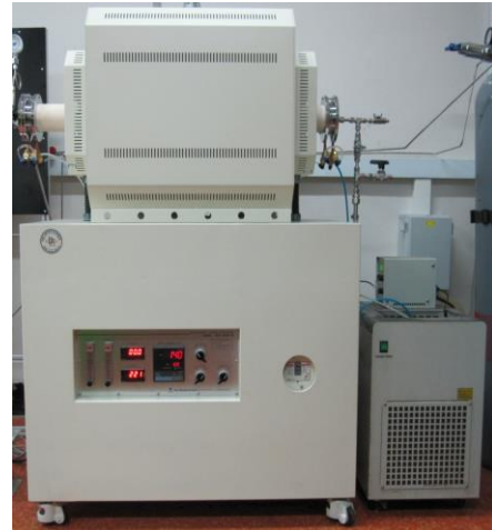
Figure 5. Apparatus (tube furnace) for high temperature oxidation of coated Zr alloys in steam
