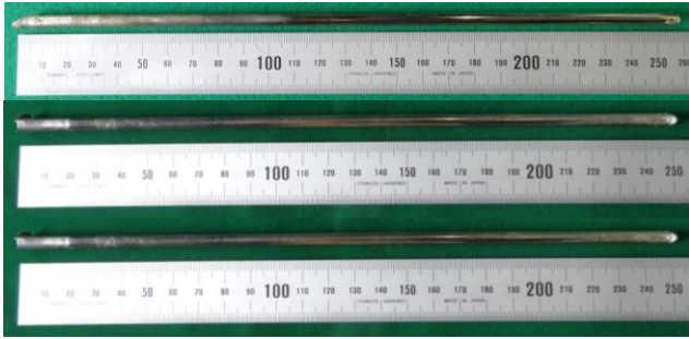
Fig. 1. Output U-10wt.%Zr-5wt.%Mn fuel slugs fabricated by improved casting method; (a) vacuum, (b) reduced atmosphere, and (c) inert atmosphere.
