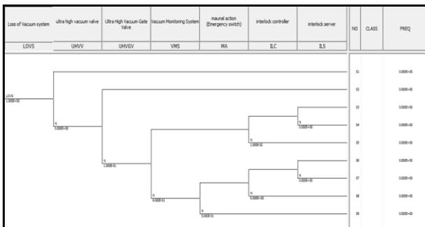
Fig. 6. Loss of Vacuum System
