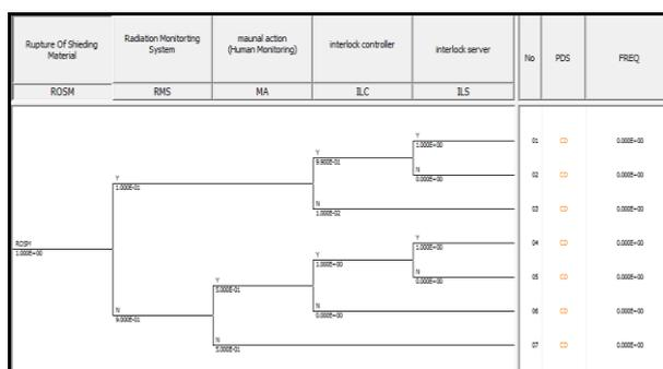
Fig. 4. Rupture of Shielding Material
