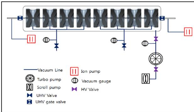
Fig. 5. Schematic of Vacuum System
