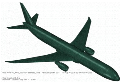
Fig. 2. Developed finite element model of large civil aircraft.
