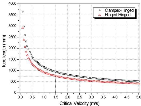
Fig. 5 Tube length with respect to a variation of the Critical velocity
