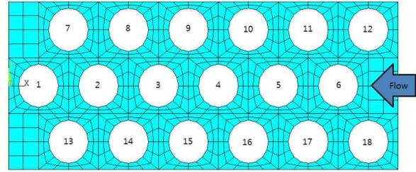
Fig. 3 The FE model of IHX tube array for FAMD code
