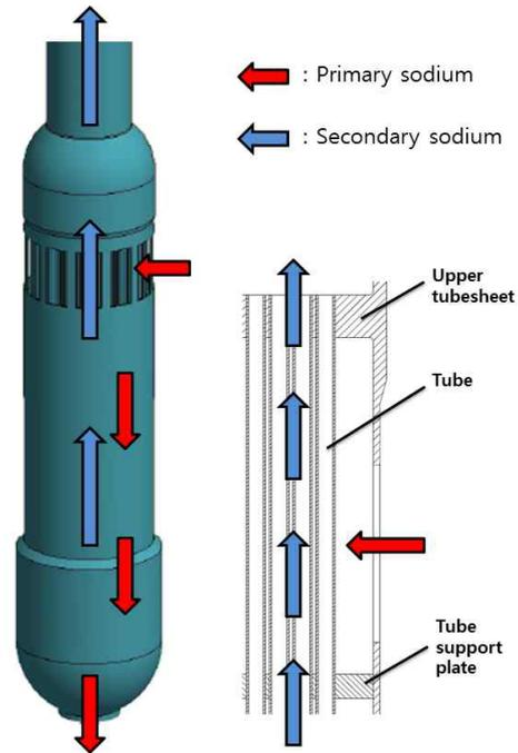
Fig. 1 a shape of IHX and flow direction of sodium
