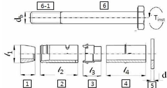
Fig. 1 Components of the anchor considered in this research
