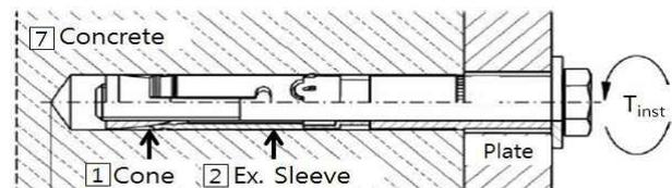
Fig. 2 Schematic diagram of the anchor-concrete contact
