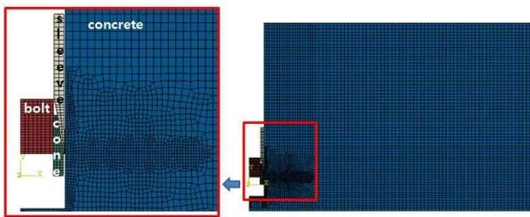
Fig. 3 FEM modeling of the anchor and concrete
