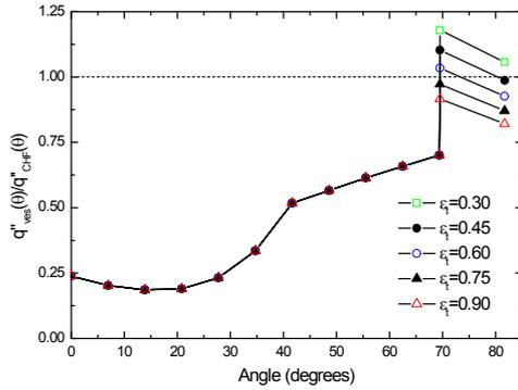
Fig. 4. Comparison of CHF ratio with light metal layer surface emissivity
