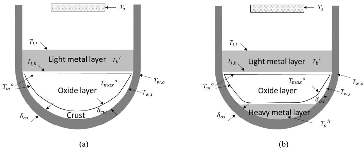
Fig. 1. The schematic of melt pool configuration (a) two layered system (b) three layered system
