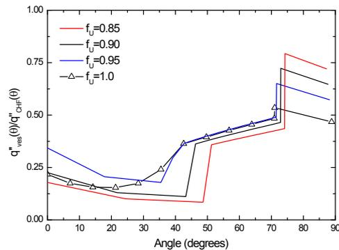
Fig. 6. Comparison of CHF ratio with fraction of uranium in the oxide layer
