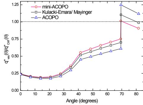
Fig. 5. Comparison of CHF ratio with heat transfer correlation of the oxide layer
