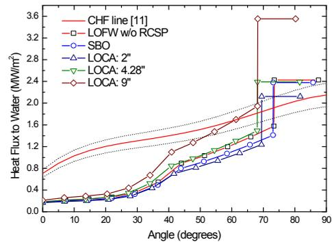
Fig. 3. Heat flux distribution based on SCDAP/RELAP5
