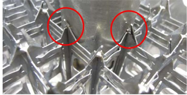
Fig. 5 Laser welding positions between SGs and a GT.
