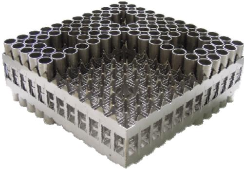
Fig. 3 A SG with modified H type springs and fuel rod mockups.
