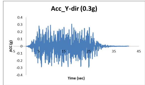
Fig. 4. Input seismic acceleration
