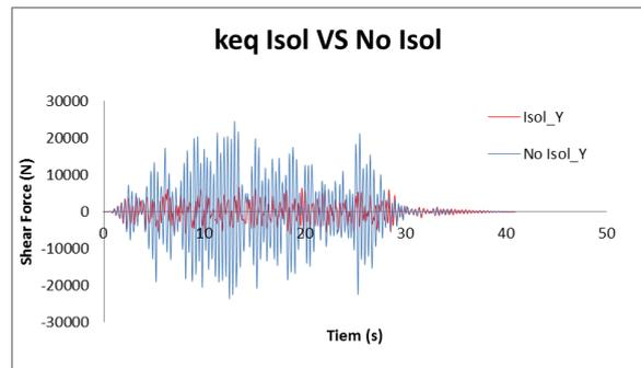
Fig. 5. The shear force of lower point of the structure
