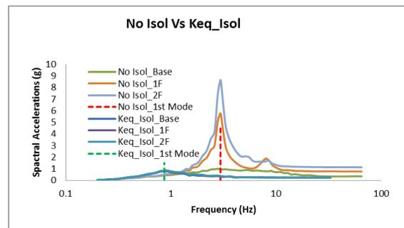
Fig. 6. The floor response spectrum of a structure
