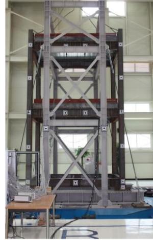
Fig. 1. The seismic base isolation system for shaking table test
