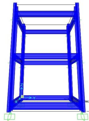
Fig. 2. The analysis model structures for shaking table test
