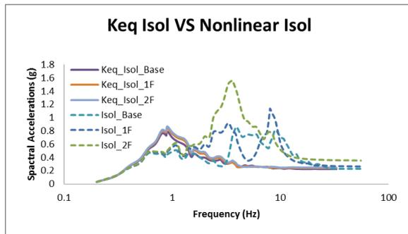
Fig. 8. The floor response spectrum of the structure in consideration of linear/non-linearity of structure
