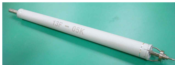
Fig. 2. The irradiation test capsule for HAMP-1
