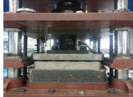
Fig. 1. View of the LRB seismic isolation device
