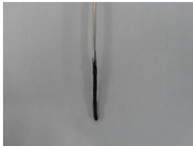
Fig. 2. Photograph of the prepared magnetite electrode with Pt wire.
