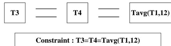
Fig. 5. Constraint for Case II (measurement redundancy)
