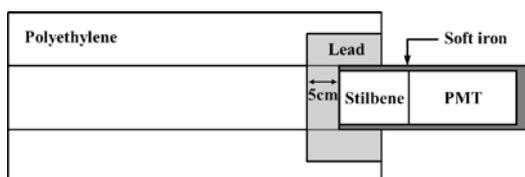
Fig. 1. Design of stilbene detector used in 2013 KSTAR campaign.
