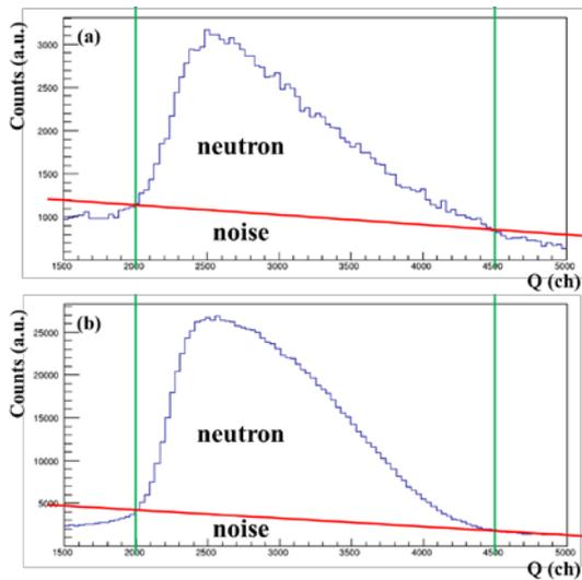
Fig. 3. Neutron spectrum in (a) 2012 and (b) 2013 KSTAR campaign.
