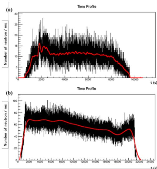
Fig. 4. Time profile in (a) 2012 (b) 2013 KSTAR campaign.
