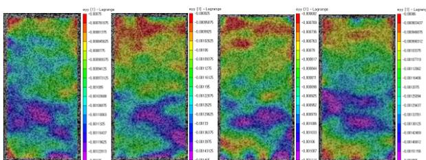
Fig. 5 Residual strain distributions after unloading to zero load at (a)  $0.35P_{max}$ , (b)  $0.65P_{max}$ , (c)  $0.80P_{max}$  and (d)  $0.95P_{max}$ .
