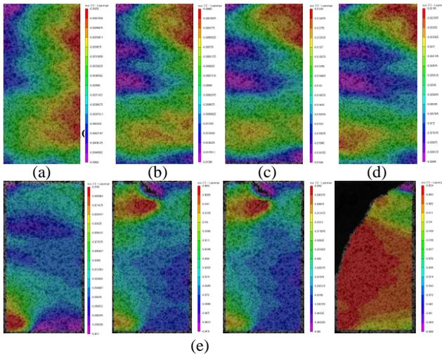
Fig. 4 Full field strain distributions at (a)  $0.35P_{max}$ , (b)  $0.65P_{max}$ , (c)  $0.80P_{max}$ , (d)  $0.95P_{max}$  and (e) near  $P_{max}$ .
