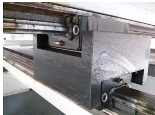
Fig. 8. Sliding bearing of excitation table
