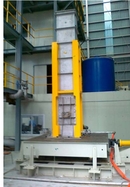
(a) Seismic test rig on exciter
