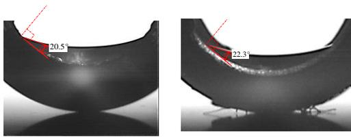
Fig. 3. Static contact angle of FC-72: (a) bare surface; (b) nanoparticles-coated surface.
