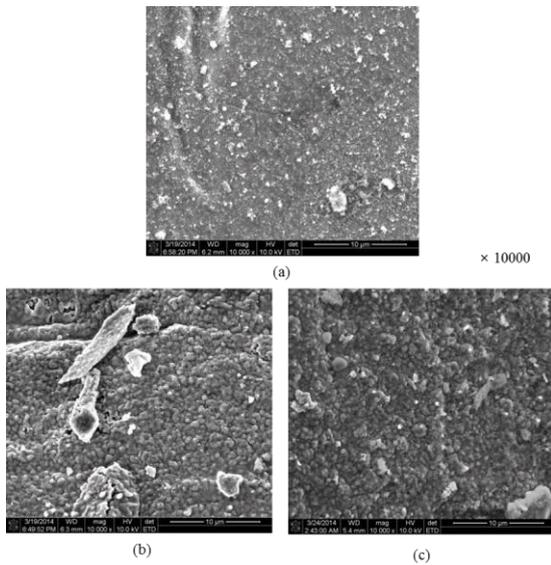
Fig. 2. SEM images of heater surface: (a) bare surface; (b) nanoparticles-coated surface before experiments; (c) nanoparticles-coated surface after experiments.
