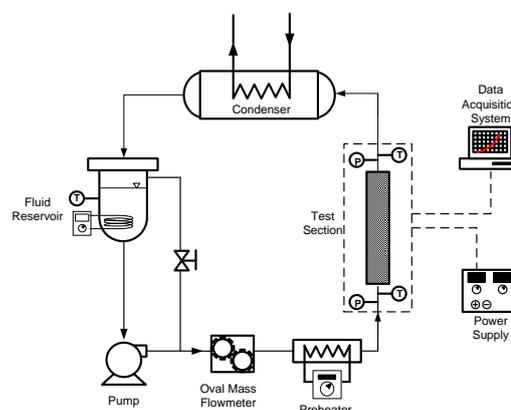
Fig. 1. Schematic diagrams of flow boiling loop
